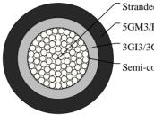
Stranded Tinned Copper Conductor 5GM3/HM3 Rubber Outer Sheath 3GI3/3GJ3 Rubber Insulation Semi-conducting Layer
